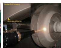
Centrifugal Pump Impeller Repair
