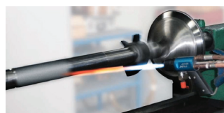
Valve Spindle Reconditioning
